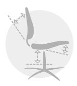
With a 3-lever mechanism the seat and backrest angles are adjusted separately and can be moved to a position that suits you and then locked in place.
