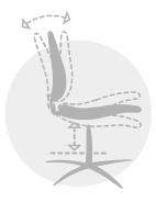
With a synchro mechanism the backrest and seat tilt movement is synchronised so they move together when adjusted. It is designed to be used in floating tilt mode so the backrest and seat move with you, following your movement to support you as you work.
